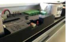
Electronic board with microprocessor, compliant with the EN16005 standard, providing direct basic programming via buttons or advanced programming via digital selector.
